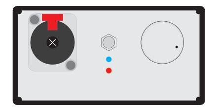
$\ensuremath{\mathsf{PPA}} + \ensuremath{\mathsf{battery}}$  board, both LEDs showing, bass boost switch.
